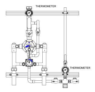
Valve assembly is certified to meet Low-Lead requirements of wetted surface area containing less than 0.25% lead by weight. All other fittings and components, the sum total of which comprise the wetted surface of this product contain less than one quarter of one percent of lead by weight.
